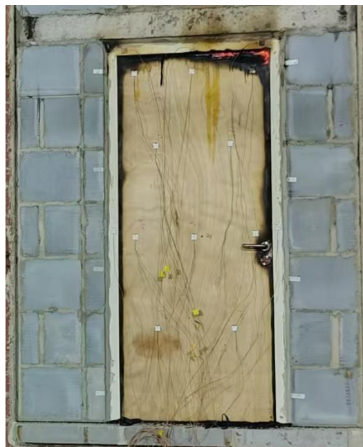
Fig. 8 Unexposed Side after 180 Minutes
