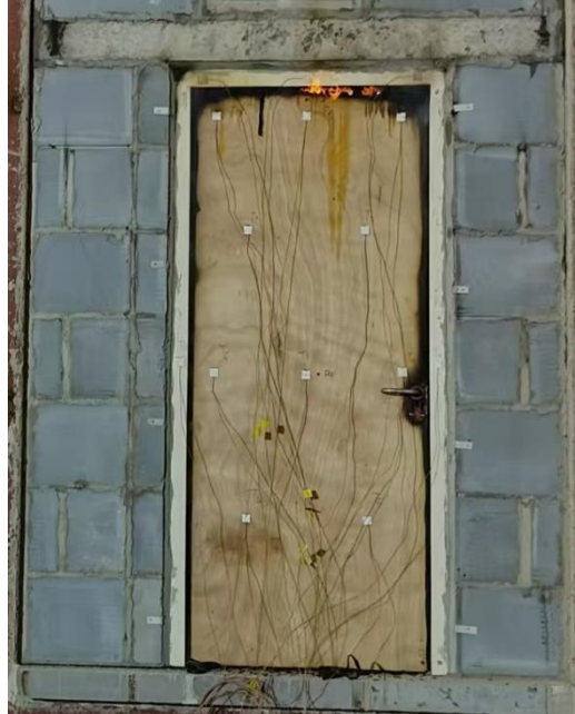
Fig. 7 Unexposed Side after 172 Minutes
