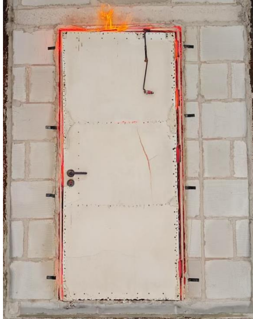
Fig. 9 Exposed Side after 180 Minutes
