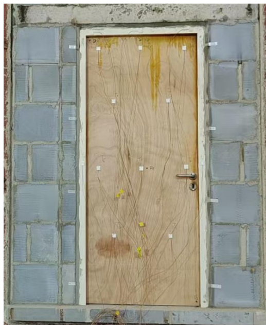
Fig. 4 Unexposed Side after 60 Minutes
