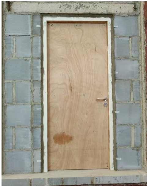
Fig. 2 Unexposed Side Prior to the Fire Test
