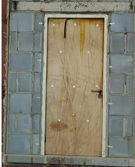
Fig. 5 Unexposed Side after 90 Minutes
